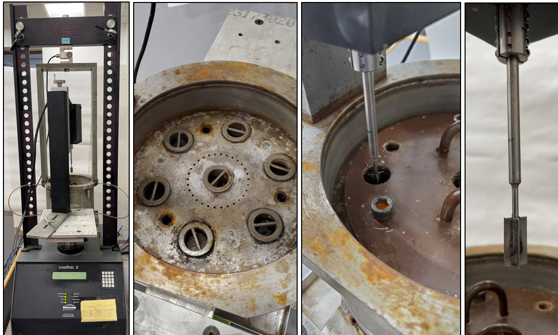
Figure 2. Photographs of Laboratory Vane Shear Testing Equipment
