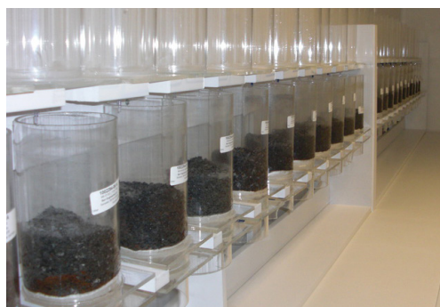
Barr designed and implemented a waste characterization plan, including humidity-cell testing and geochemical modeling, for waste rock at a proposed mine.
