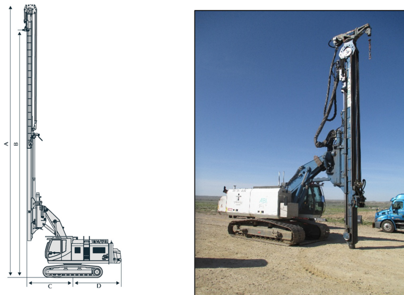
Figure 4. ABI Pile Driver
